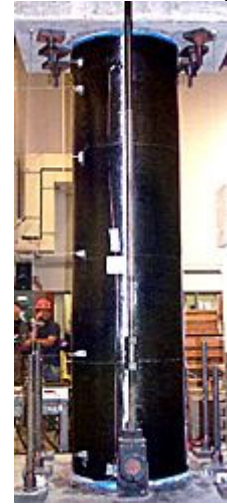
Photo: 3 Completed Laying with Build Seal Prepreg
